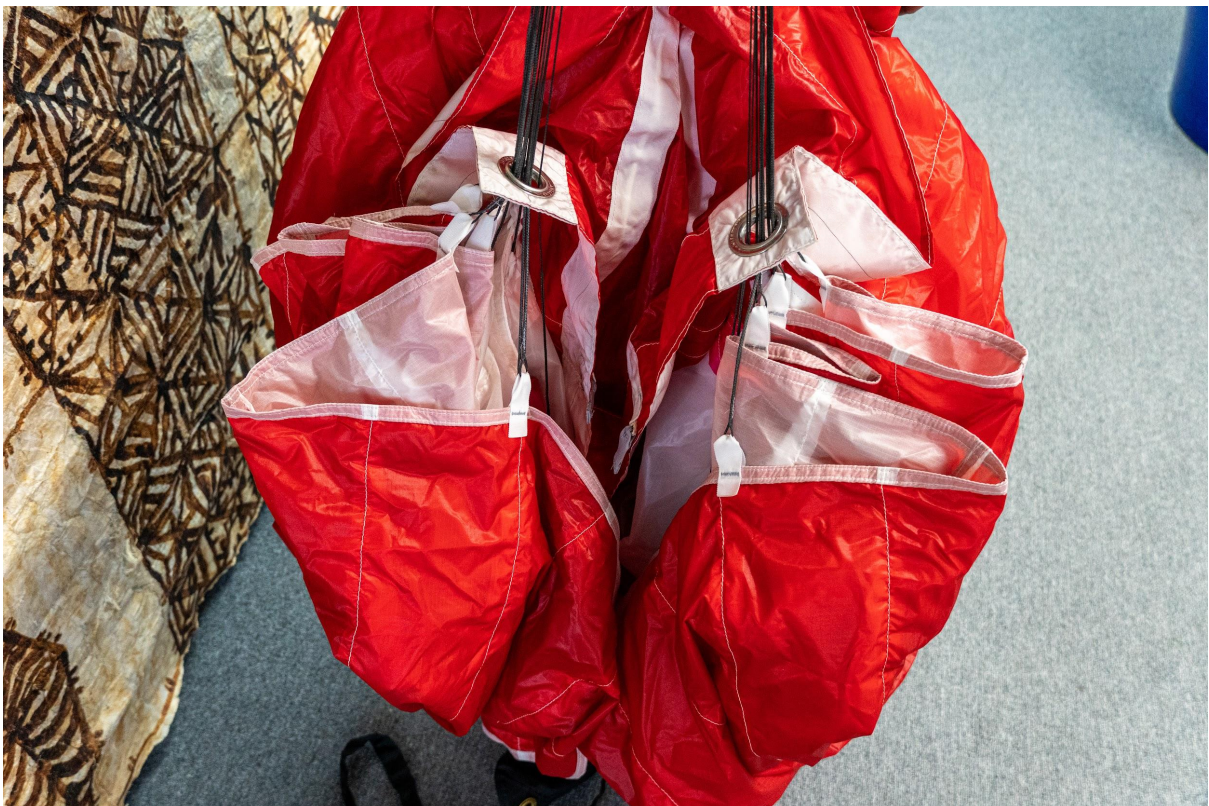
Flaking out instead of in will help to keep lines centered.
