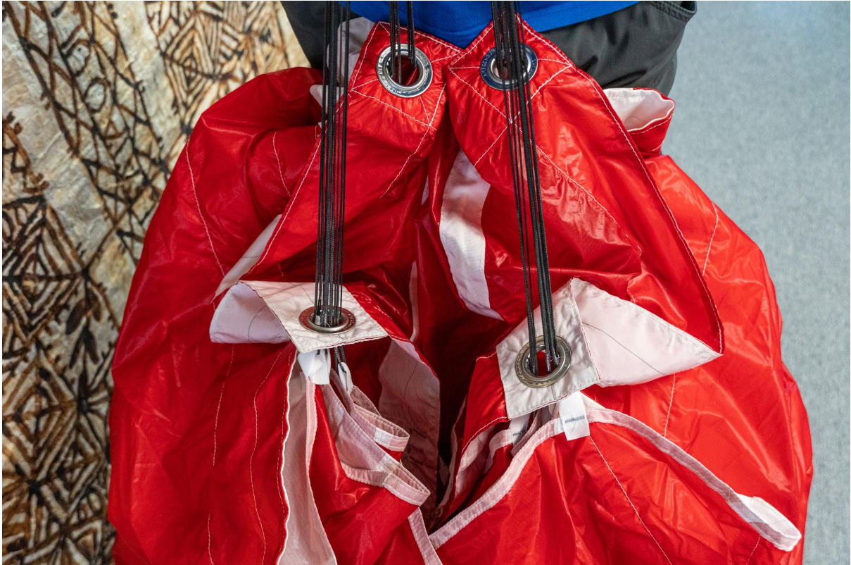
Flared slider to control outside material.
