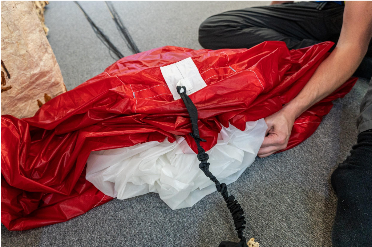
Pull top skin to tidy line slack. Be careful not to pull excessively, it can increase the problem
