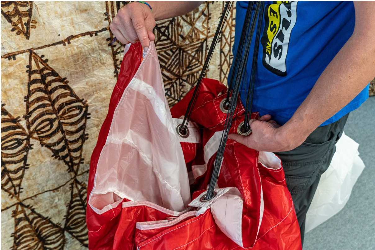
Tail lifted to high past grommets
