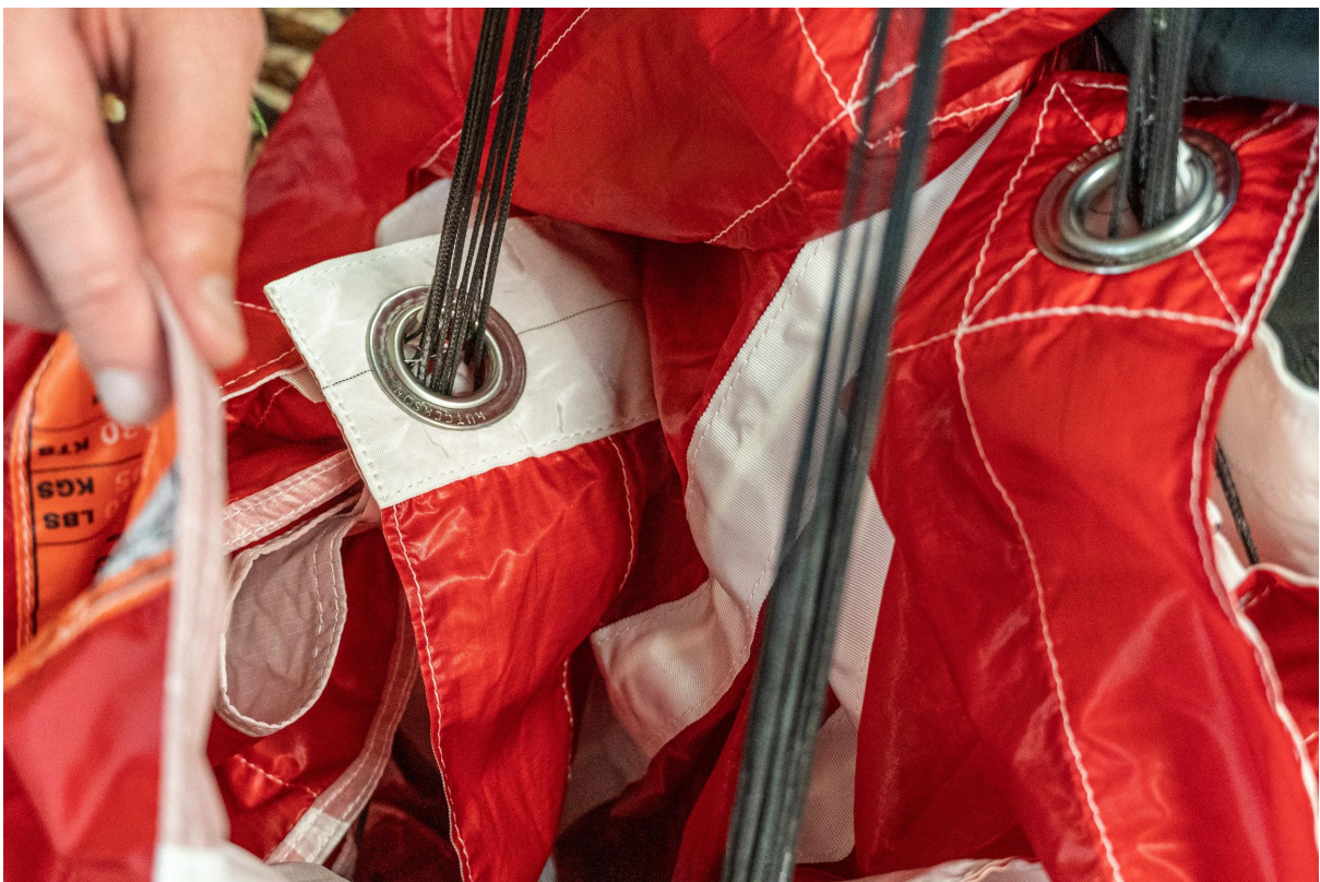
No unnecessary slack lines
