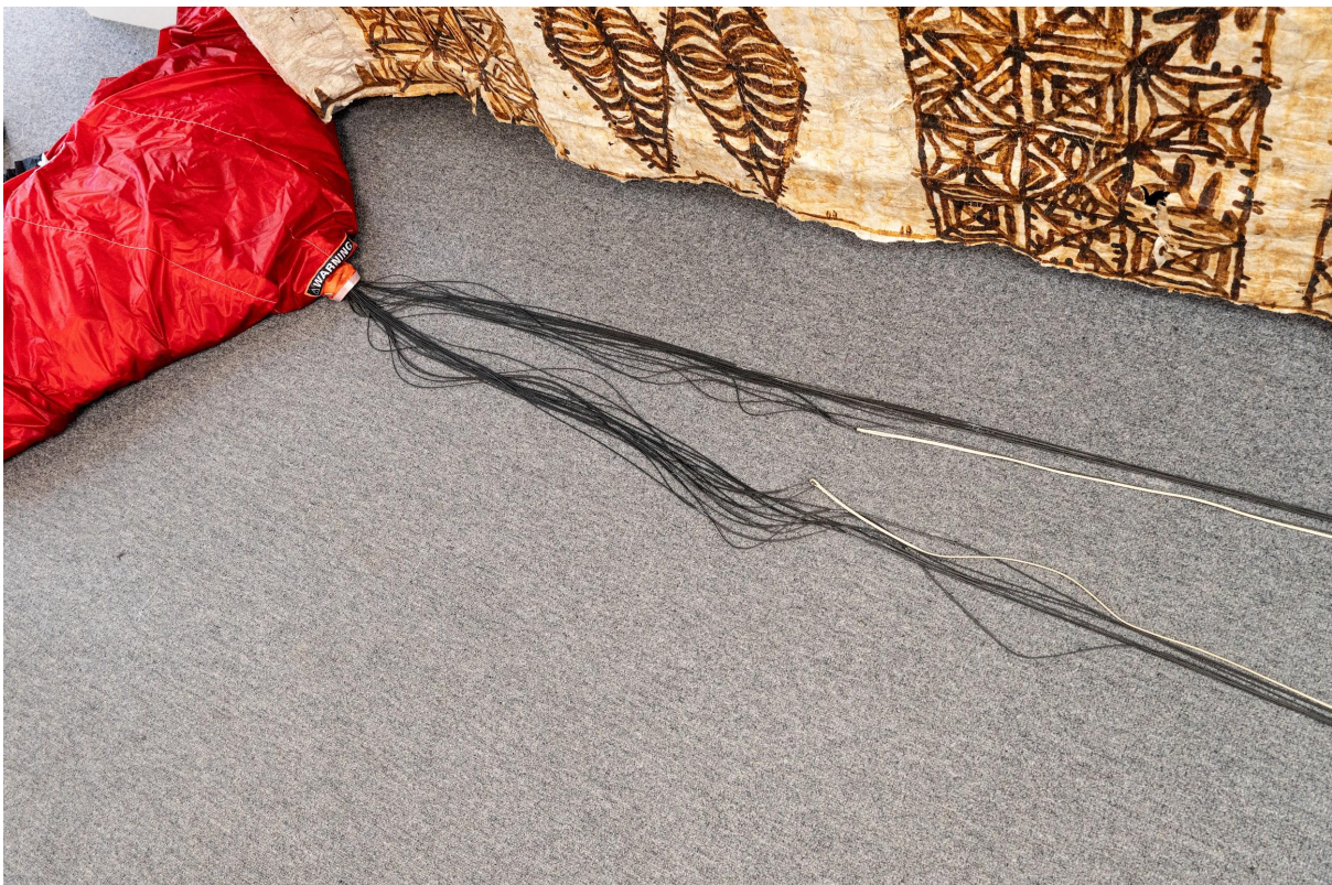
Excessive slack, start pack job again
