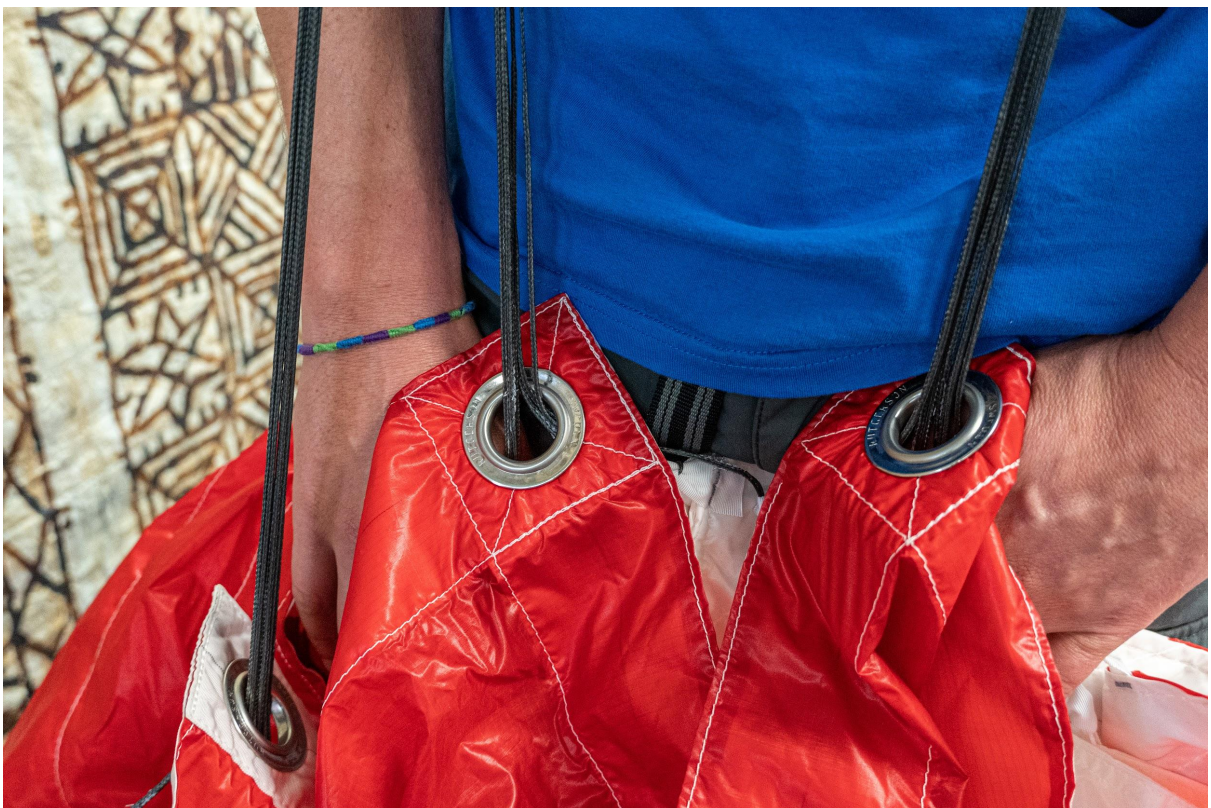
Correct tension with no slack lines
